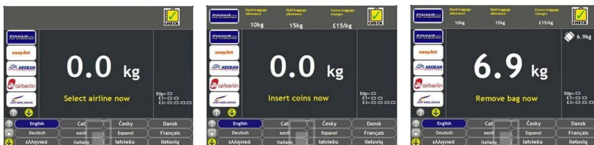
If the passenger inserts £1 or £2 (€2 in Eurozone), multiple bag weighs are offered. After the first bag is weighed the weight is recorded in the right hand side of the screen and the passenger is invited to put the next bag on the scales. The machine detects the second bag and displays its weight, recording it on the right of the screen just below the first bag's weight. Further bags can be weighed in this way until the full value of the coins has been used up.
